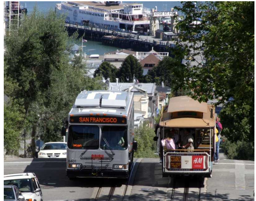
2006 Orion VII hybrid bus meeting a cable car at the top of Hyde Street - a 21% grade
