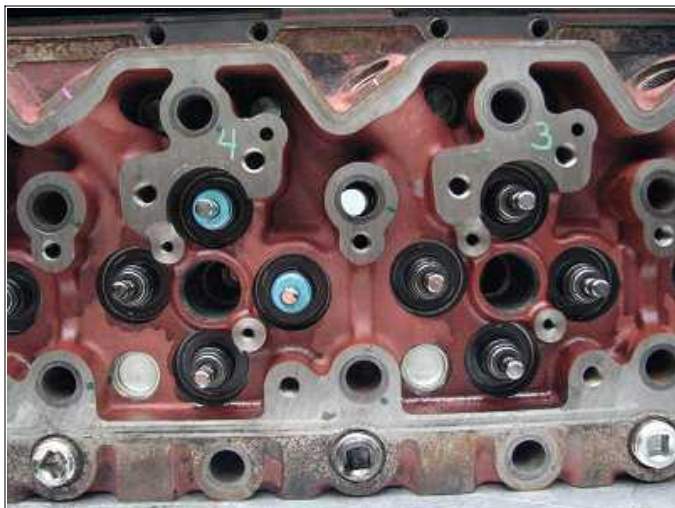
Top of cylinder head No sludge deposits
