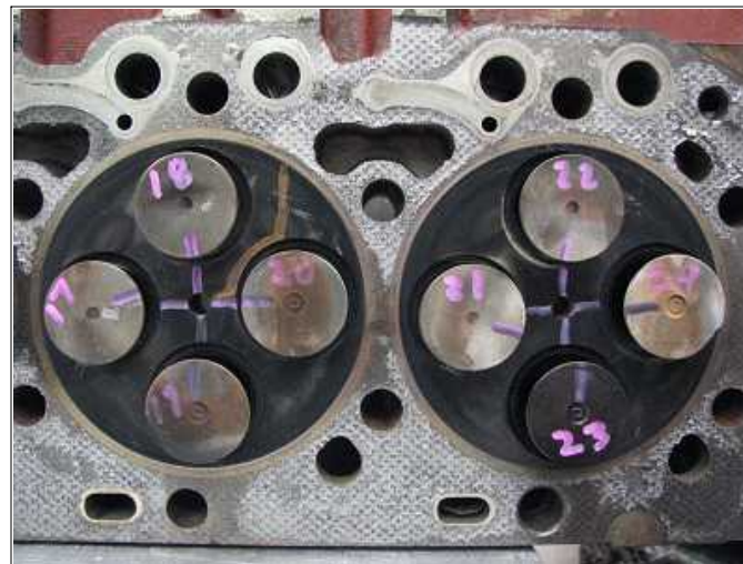
Bottom of cylinder head Deposits comparable to #2D
