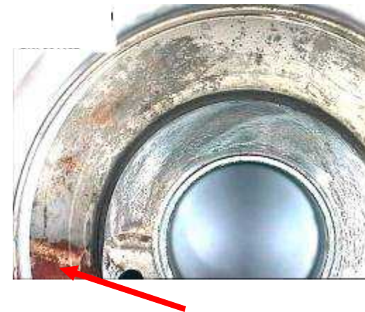
Fuel pump hsg deposits and corrosion from low use test
